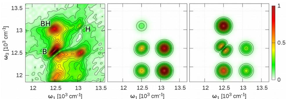
Fig. 1. All-parallel oscillation map at 560 cm<sup>-1</sup>. Left: experimental oscillation map of rephasing real 2D signal, center: modeled pattern expected from normal stimulated emission and ground state bleach contributions, right: modeled interference between ground state bleach and ETICS signals reproducing cancellation on the diagonal.
