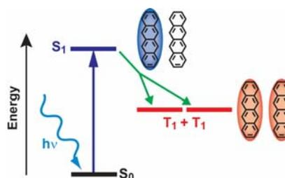
**Figure 1:** SF materials can prepare two electrons from a single photon by generating triplet pairs.
