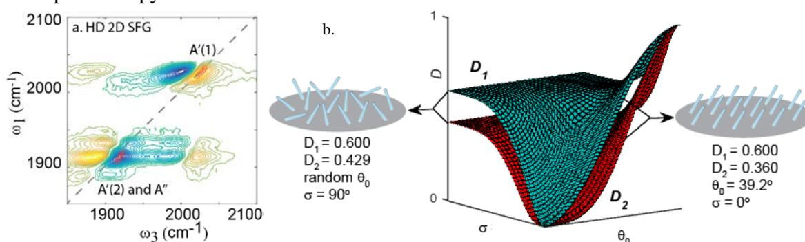
**Figure 1. (a) HD 2D SFG spectrum of Re(diCN-bpy)(CO)<sub>3</sub>Cl on gold surface. The center-line-slope indicate that A'(2) mode has stronger interactions with the surface than A'(1) mode. (b) by determine two independent orientation parameters, the mean orientation and orientation distribution of an ensemble averaged monolayer can be unambiguously determined.**
