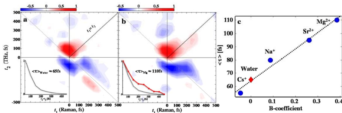
**Fig. 1** a) The experimental 2D Raman-THz signal of a) water and b) 2M  $MgCl_2$ . Insets display the cuts along the diagonal  $t_1=t_2$ . c) Relaxation times for the series of 2M  $X^{n+}Cl_n$  salts vs. Jones-Dole  $B$ -coefficients.
