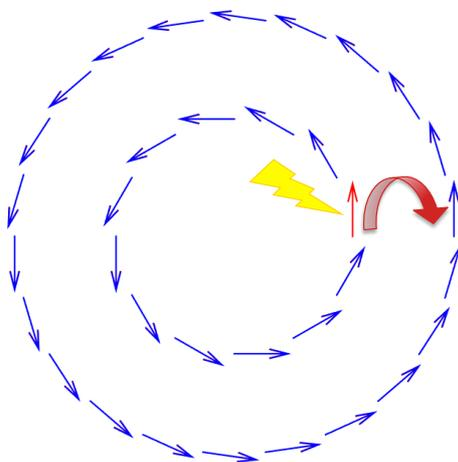
Fig.1 Phenomenological model of a coupled ring system, where blue arrows represent transition dipole moments of the chromophores lying in the plane; the red arrow represents an initially excited chromophore. The comparison of methods is based on the study of the excitation energy transfer rate from the inner ring to the outer ring.
