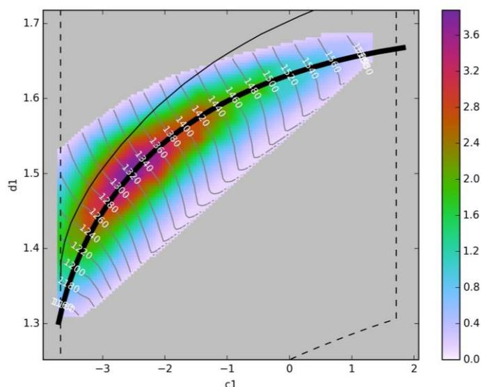
**Fig.1** Automatically generated plot of typical fs OPA preamp tuning acquisition. Axes are OPA motor positions, with dotted lines indicating scanned motor position range. At each motor position the spectral OPA output is fit to a Gaussian. After filtering for good fits, the amplitude (colorbar) and central color (grey contours) of the fit outputs are plotted. Also shown: the previous tuning curve (thin black line) and generated tuning curve (thick black line).
