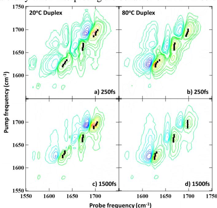
Figure 1 – 2D-IR spectra of AT 15mer duplex recorded at 20°C (a,c) and 80°C (b,d) at early and late waiting times. At low temperatures in the double stranded helix, little to no spectral diffusion is observed as Watson-Crick hydrogen bonds prevent solvent access. At elevated temperatures, when the duplex has been denatured into component single strands then spectral diffusion of the diagonal modes is observed due to increased solvent access.
