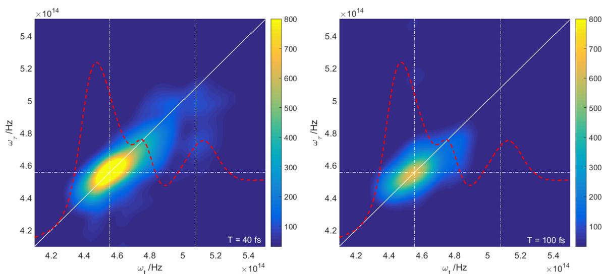
Fig 1: Absolute 2D spectra of Pentacene films at 40 fs and 100 fs population time. The peaks at 520 THz are absent in the 100 fs plot. Static absorption spectra are shown in red.
